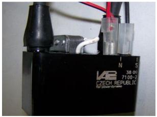
The wider, 6,3mm pin shall connect to the red/white wire that brings the ignition voltage.
