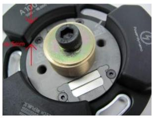
Place the adapter onto the engine. The wire opening of the adapter will show to about 2 o'clock. Screw the adapter down with the 3 countersunk screws M6x25.
