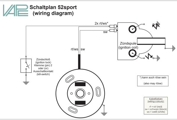
Screw the high tension cables into the ignition coil and place the rubber seals over the exits. It's more easier if you do that before mounting the coil. Please do use the cable arriving with the pack and not any old cables.
