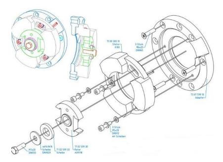
Please ensure that all parts supplied are installed. It is important that the 3 large washers are placed onto the rotor, as otherwise fastening of the rotor ist not possible.
